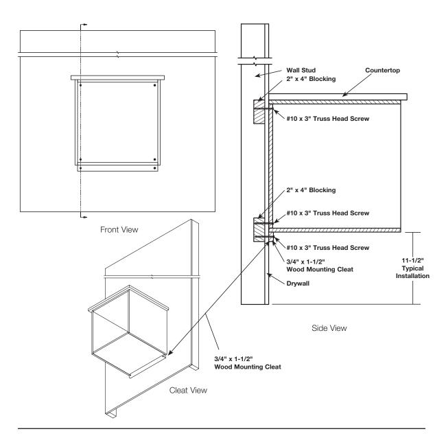
• Floating vanities have a weight limit of 300 lbs. (including countertops) when installed properly
